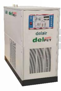
Delair has specially designed Delpet Compressed Air Dryer for PET Bottle manufacturing process. It operates at high pressure upto 40 bar on the method of cooling the air to near freezing point to remove the moisture and reheating it to approximately 10°C below the incoming compressed air temperature at nominal conditions.
